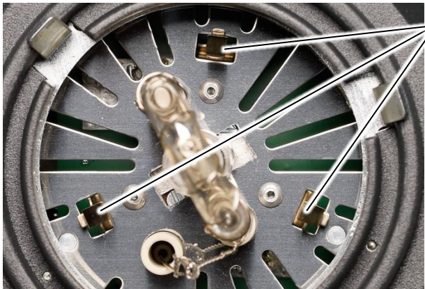
Springs holding the glass safety dome
