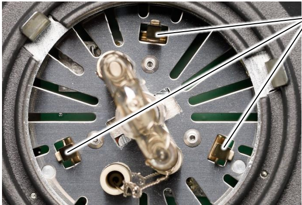
Springs holding the glass safety dome
